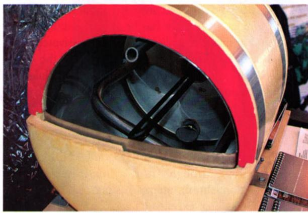
Top: The heat exchanger inside this water heater transfers heat from the engine coolant to domestic water. The "fins" increase surface area to improve efficiency and reduce the time required to heat the water. Above: Where water heater insulation is concerned, more is better. This cutaway reveals ample insulation, particularly in the upper section of the heater's tank. Because heat rises, it is especially important to keep this area well insulated.
